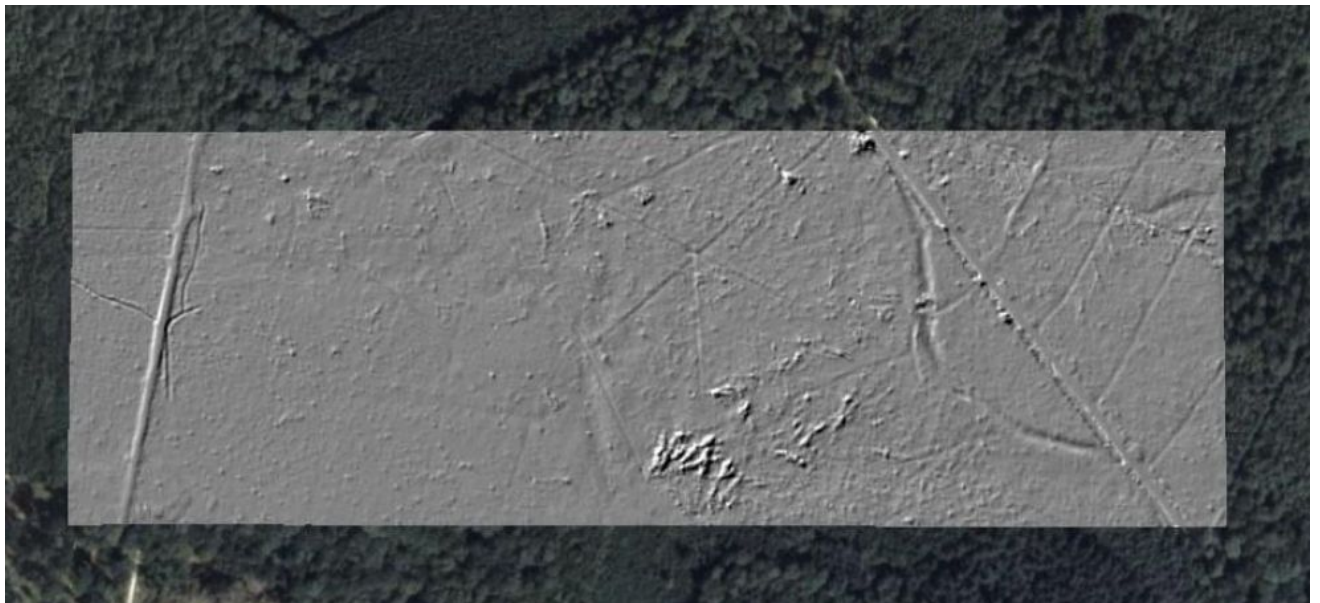
Fig. 3: DTM (grey rectangle) with Orthophoto in the background. Hidden features under the canopy become visible, such as roads and logging lines.
